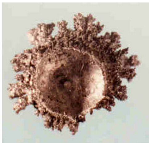
Figure 3. The result of GaN synthesis from the liquid Ga and N 2 plasma. The liquid has been pushed out from the initial droplet covered by GaN crust by the growing N 2 bubbles.
